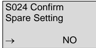
After selecting YES, the FWD and REV LEDs turn off (for SINUS PENTA only), and three dashes (---) appear instead of "NO" on page S024. This means that the Penta drive is ready to start.
